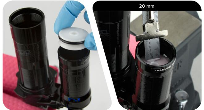
**8** Continue to cover the damper body with your hand and install a new bleed screw into the bleed port. Tighten the bleed screw until the IFP begins to spin.
