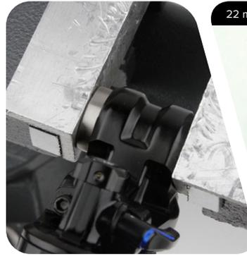
22 mm (OD) x 10 mm (ID) bearing press tool
