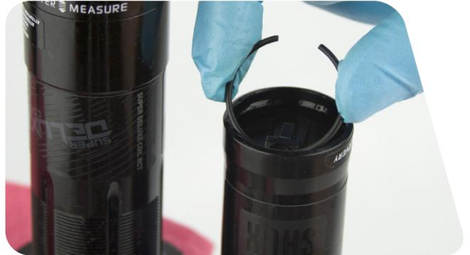
**20** Pull up on the IFP reservoir cap to seat it against the retaining ring.
