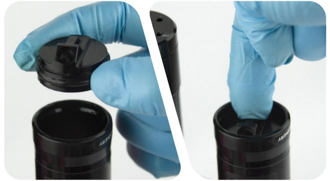
**19** Push the new retaining ring into the groove until it is seated.
