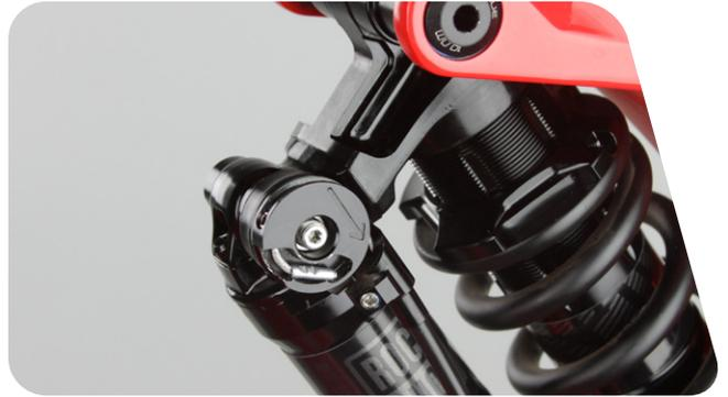
**5** Install the cable spool cap and tighten.
