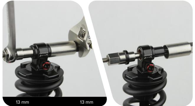
**4** If the bushing pin did not remove easily, unthread the push pin from the threaded rod to remove the end spacer, then reinstall the push pin onto the threaded rod.
