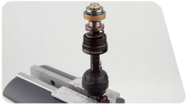
**13** Remove the main piston nut. Clean the nut and the threads of the shaft assembly to remove all traces of Loctite.
