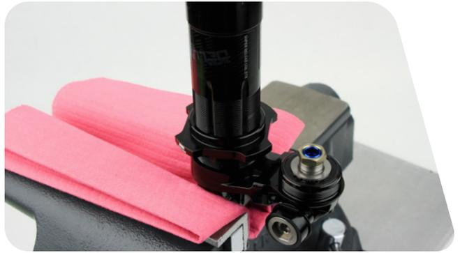
**4** Thread the IFP reservoir onto the eyelet. Tighten the IFP reservoir.
