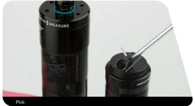
**7** Remove the IFP reservoir cap o-ring.
