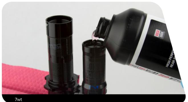
**6** Once most of the oil from the IFP reservoir has moved to the damper body, use the palm of your hand to tap down on the top of the damper body repeatedly to move oil back into the reservoir. This will further assist in purging air bubbles from the system.
