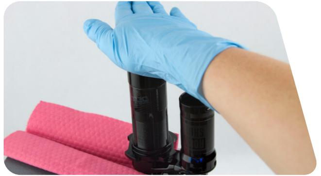
**7** Install the IFP into the damper body with the flat side visible. Use a metric caliper or ruler to push the IFP into the reservoir to a depth of 20 mm.
