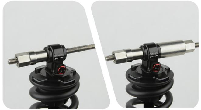
**3** Hold the catcher secure with a 13 mm open end or adjustable wrench.
