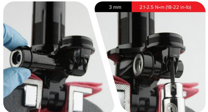
**14** Install the lock spring and lock shim into the reservoir mount.
