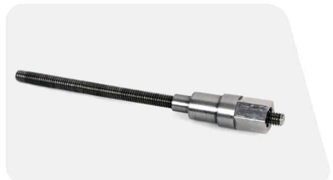
**2** Insert the threaded rod through the shaft eyelet until the push pin rests against the bushing pin.
