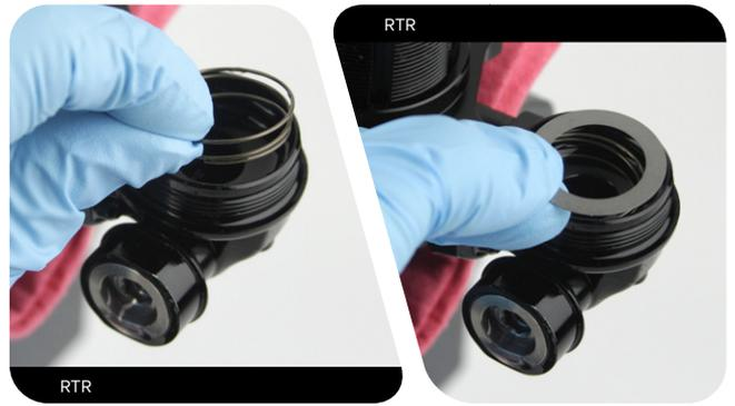
**15** Install the compression assembly into the reservoir mount. Push the compression assembly into the reservoir until it stops.
