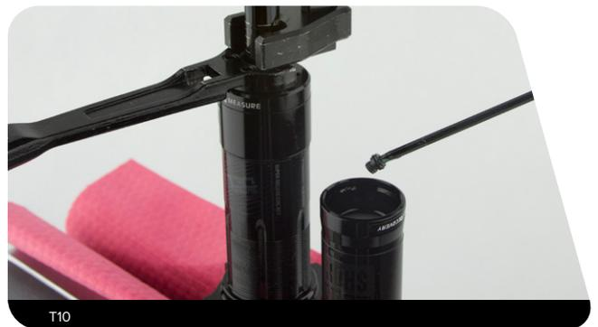
**12** Place a shop towel around the IFP reservoir to catch oil overflow. Insert a small hex wrench through the slot next to the 33 or 39 mm mark on the IFP Height Tool, depending on your shock stroke.
