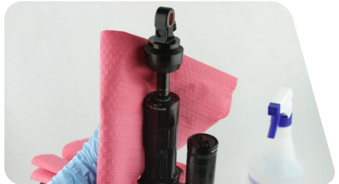
**28** Install the coil spring and spring retainer.
