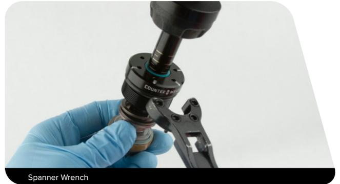
**2** Assemble the Counter Measure Compressor so that stop 1 is at the end of the shaft, then tighten stop bolt 1.
