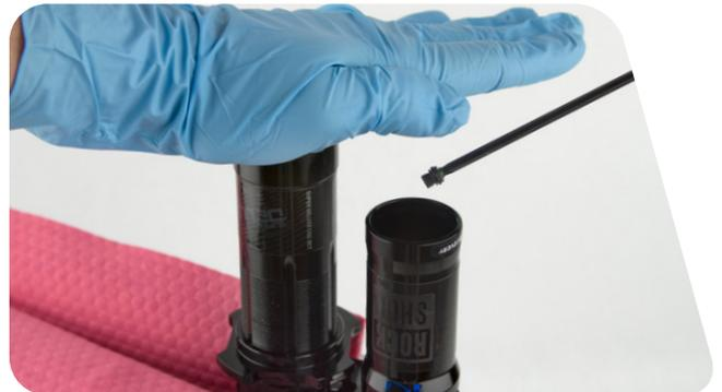
**9** Pour additional oil into the damper body until the oil is level with the top of the threads.
