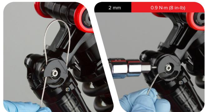
**4** Trim the cable, install an end cap, and tuck the cable into the pocket.
