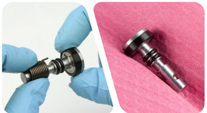
**8** Apply a thick layer of grease to the cam.
