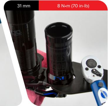
**5** Pour suspension oil into the IFP reservoir until it is level with the top of the IFP reservoir. Oil will begin to bleed into the damper body.
