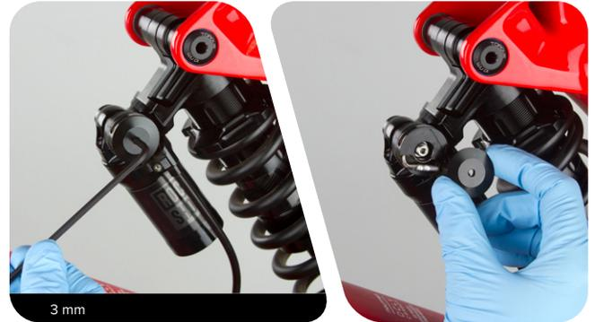
**2** Loosen the cable set screw, then cut the cable.
