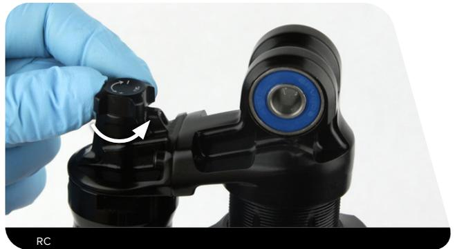
**2** Turn the preload adjuster counter-clockwise until there is a large gap between it and the spring.
