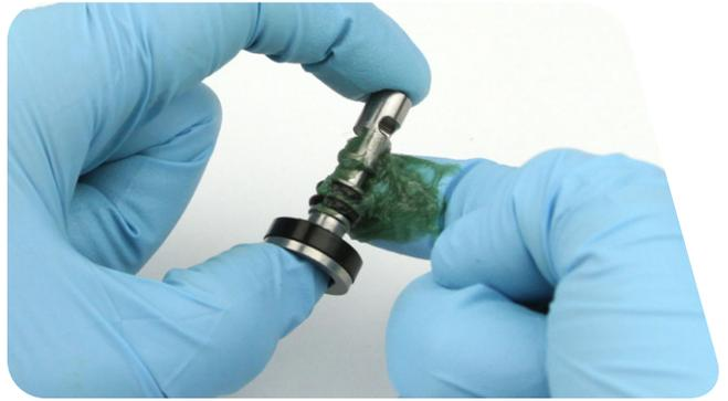
**9** Apply a thick layer of grease to the inside and outside of the new remote spring, then install the spring onto the cam with the spring tang in the spring tang hole.
