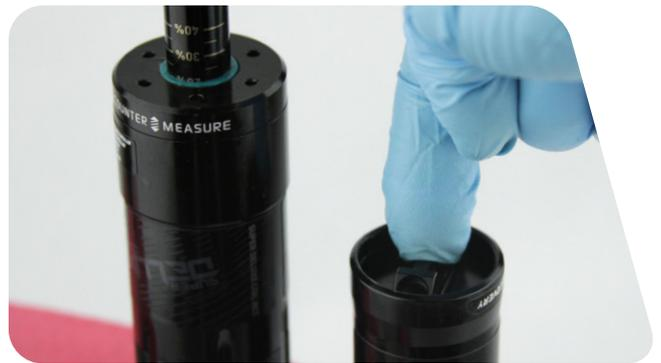
**5** Remove the retaining ring from the IFP reservoir.
