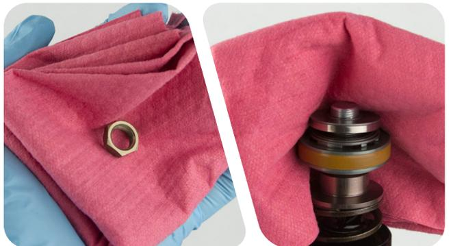
**14** Slide the main piston assembly and top out plate off the shaft and onto a small hex wrench or pick.
