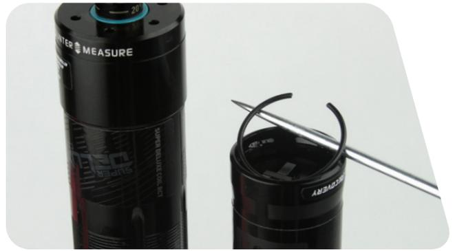
**6** Remove the IFP reservoir cap from the IFP reservoir.
