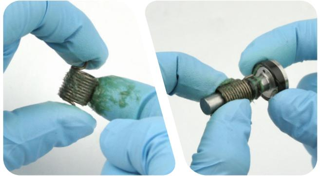
**10** Install the cam and spring into the cam housing, and rotate the cam until the spring tang falls into the tang hole. The cam should be flush with the end of the cam housing.
