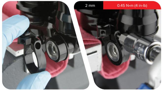
**26** **RTR:** Install the cable spool onto the cable hanger with the arrow pointing at the cable hanger, then tighten the remote screw.
