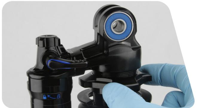
**3** Remove the spring retainer and spring.
